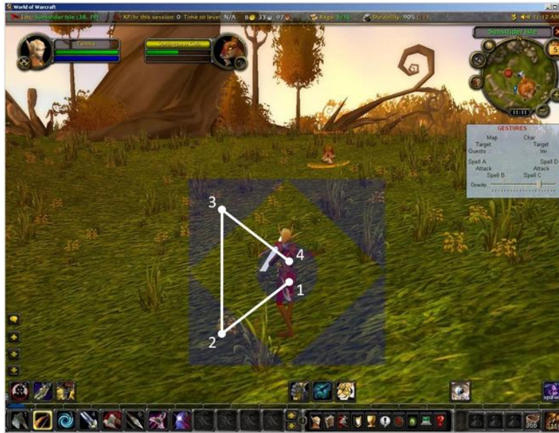
Fig. 1. Twelve gestures are supported, each of which can be assigned its own keyboard or mouse event. A gesture is produced by looking from the centre zone to one of the four corner zones then back to the centre, either directly or via another zone.
