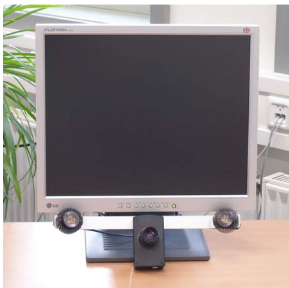
Figure 1. Remote eye tracker system setup. The eye tracking hardware consists of a single high-resolution camera below the display and two infrared LEDs to either side.
