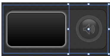
Figure 1. The Binary Choice component. Upon gaze entering the component a opaque layer expands to the right, revealing the saccade icon (2, shown as a speaker). A growing white border indicates the activation process (3). The changed/selected state is then indicated by the background of the component (4). The speed of the rollout and the activation threshold is configurable.
